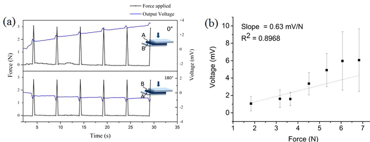
FIG. 2. (a) Piezoelectric voltage generated from a monoclinic film of lysozyme in response to dynamic force pulses when the sample is upright ( $0^\circ$ ) and inverted ( $180^\circ$ ). (b) The magnitude of the voltage generated increases with increasing force applied.
