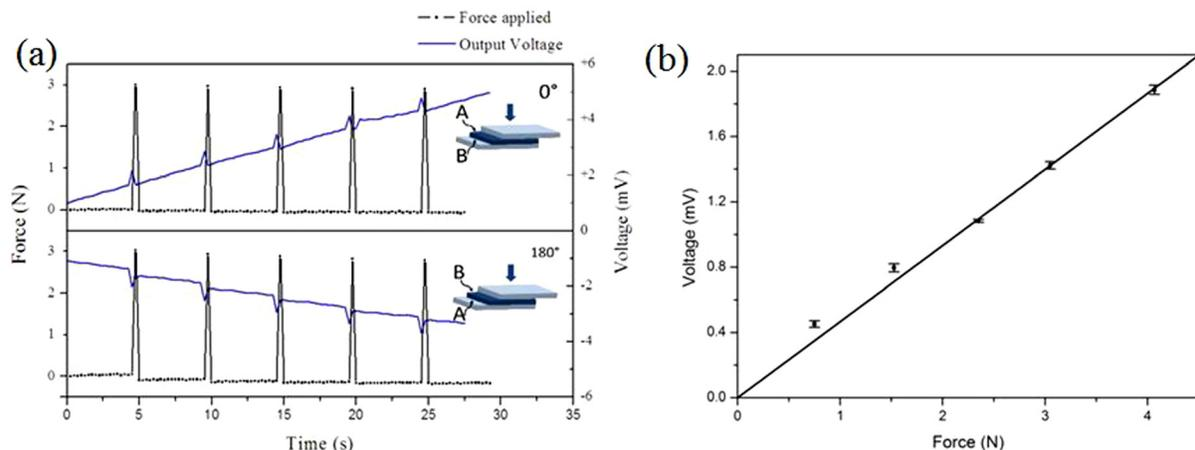
FIG. 3. Application of dynamic force pulses induces voltage peaks in tetragonal lysozyme films, which switch polarity when the sample is changed from upright ( $0^\circ$ ) position to the inverted ( $180^\circ$ ) position (b). The voltage generated increases linearly with the magnitude of force applied.
