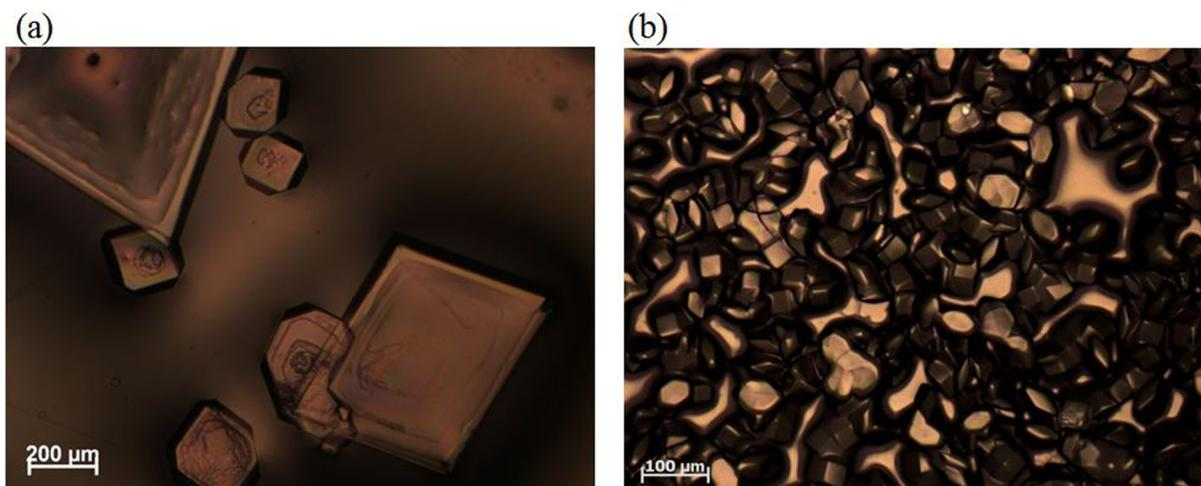
FIG. 1. Optical microscopy images of (a) monoclinic and (b) tetragonal aggregate films of lysozyme.
